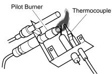
Figure 26 - Incorrect Pilot Flame Pattern
